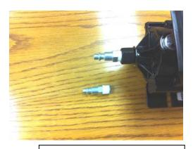
Example of a male quick disconnect Than can be used to connect the air source hose to the pump. The customer can configure the hose and pump fittings In any way they choose. This is just an example of how most customers make the connection. If using the quick-disconnects, be sure to use Teflon tape or pipe thread sealant on the threads.
