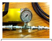
Hydraulic Pressure Gauge.connects to pump via the provided quick-disconnect fittings. If the gauge fittings are difficult to insert, connect the air line to the pump and activate the foot peddle to pressure up the pump, then release the foot peddle to relieve the hydraulic pressure. The connections should now install easily.
