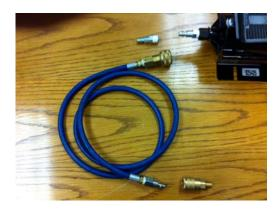
Air hose shown equipped with Quick-disconnect. Customer can Use any fittings or adaptors they Choose to connect to the pump. Quick disconnects make it easy to Separate the pump from the air hose
