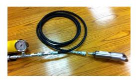
The black hydraulic hose connects To the pressure gauge and handset Via the provided quick-disconnects.
